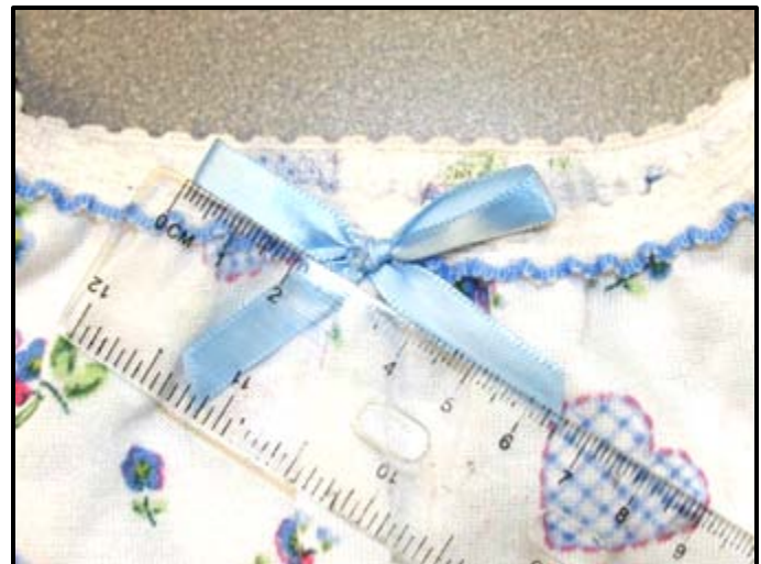
Figure 53. Test trim pieces greater than 5.18 cm in longest direction
