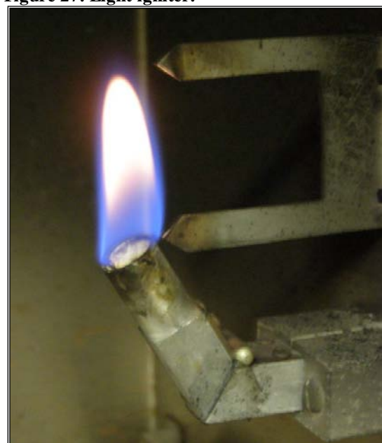
Figure 28. Check flame length.
